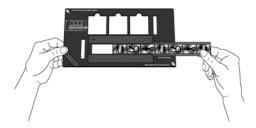
2. Place the mask on the glass so the arrow on the mask labeled **Use this mask for scanning 35mm negatives** is aligned with the arrow in the upper left corner of the scanner.
